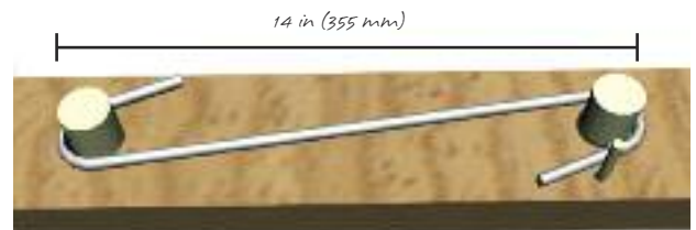
Figure 7: Stirrup Jig for Two-Course Bond Beam
