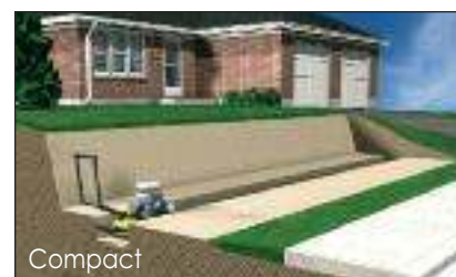
Install drain pipe, wall rock and level
